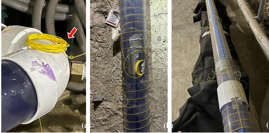
Figure 2. (a) Photograph of red laser light transmitted to the last cable, helically wrapped cable from OTDR test. (b) Photograph of extra looped cable around a splice point. (c) Photograph of loosened loops to improve signal.
