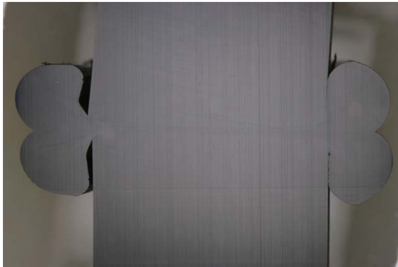
Figure 4.8. Surface of HDPE Pipe 1224, Quadrant 4 at Approximately 3.4 Inches (8.6 cm). No lack of fusion is seen.
