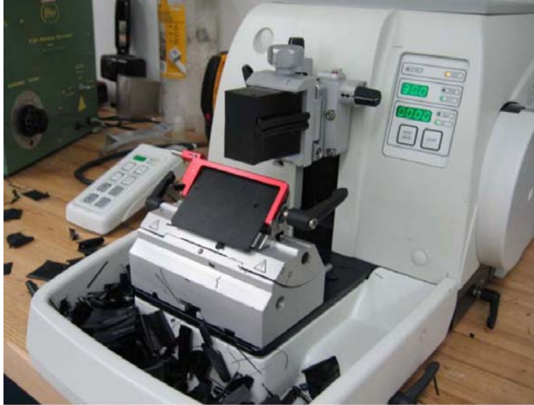
Figure 4.2. Rotary Manual Microtome Used to Slice HDPE Pipe Sections. The unit was on loan from Bartels and Stout, Inc.
