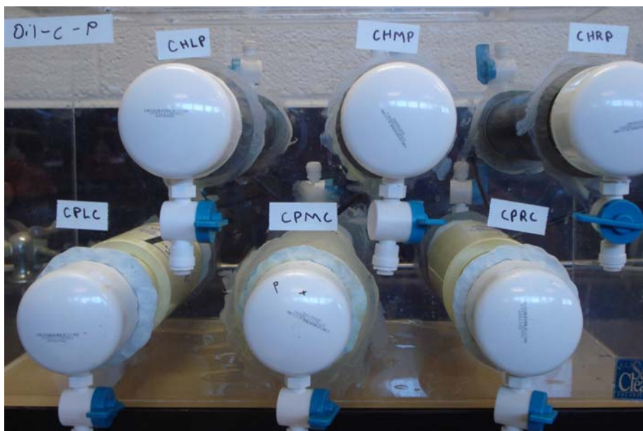
Figure 3.1. Acrylic Tank used to perform permeation study on Polyisoprene couplings and HDPE pipe using Oil-C.
